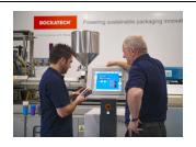
Photo: EcoCore MuCell development is carried out at the Bockatech R&D centre in the UK on a high speed BMB injection moulding machine fitted with a Trexel P-300 SCF delivery system.
