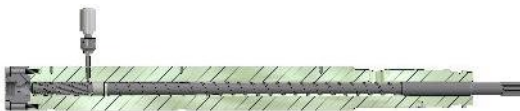
Picture: TDM-Tip-Dosing-Module.jpg Enclosure: MuCell Tip Dosing Module on a standard screw in long barrel
