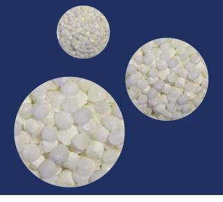
TecoCell GT chemical foaming agent is a specially formulated concentrate that is recommended for foaming PET, PETg, Nylon, PLA and other high temperature processing polymers.
